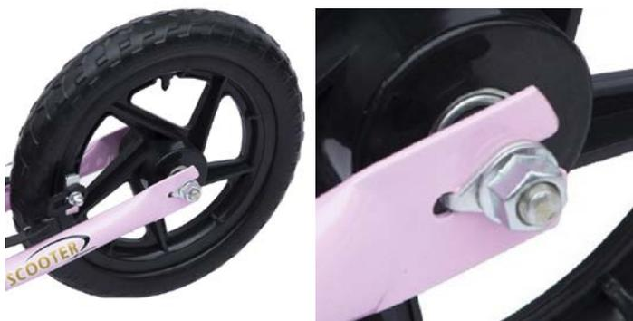
Back Wheel Push into axle slots. Install the tab washer first (a). Then install the axle nut (b) tighten with Spanner or wrench.
